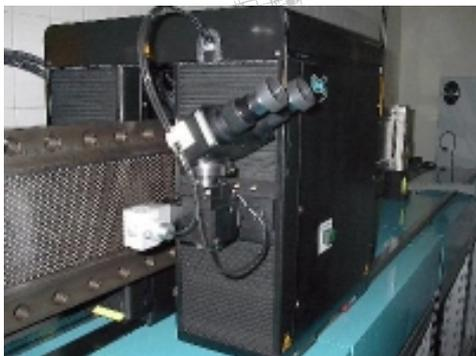
A portal construction is assembled on precise grinded linear bearings. Due to the usage of an optic linear scale, the portal can be positioned very precisely.
