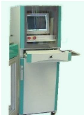
Measuring computer, motor control, printer and light sources are built in a industry usable tower case for 19" components. The cables are guided by a solid cable carrier along the linear axis.
