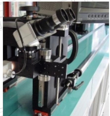
Both microscope tubes can be adjusted vertically by handwheel, gear belt and screwed spindles.
