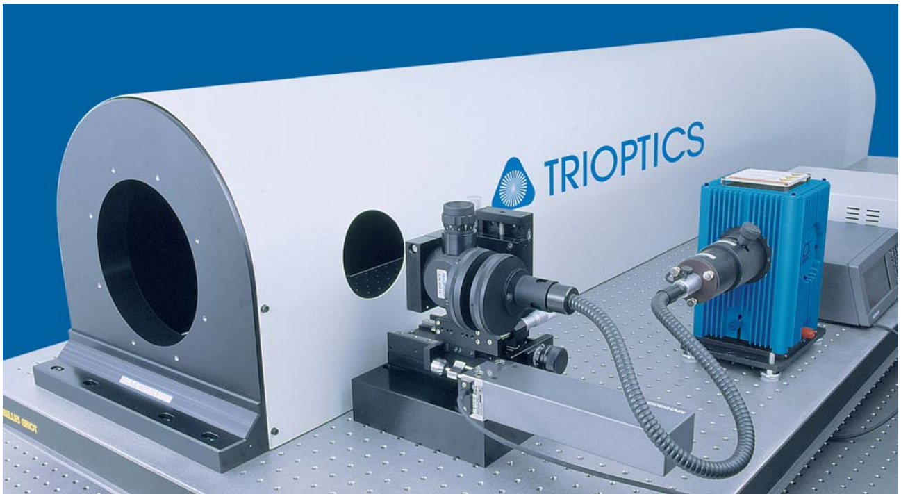
High Quality Mirror Collimator EFL 2000mm, Aperture 200mm, Surface quality: \lambda/15
