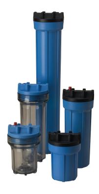
Pentair® Pentek® Slim Line® Filter Housings are available in either reinforced polypropylene or clear Styrene-Acrylonitrile (SAN) in 5", 10" and 20" lengths. The black or blue reinforced polypropylene housing caps are available with 1/4", 3/8" or 1/2" NPT connections. Four bosses are molded into every cap for mounting purposes.
