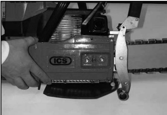
STEP 2 Mount SpeedHook® mounting bracket over bar mount studs
