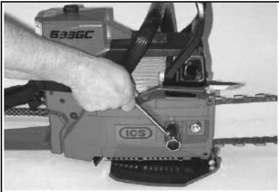
STEP 1 Remove side cover (retain side cover for future use with Wallwalker®)
