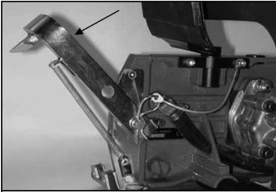
STEP 1 Remove Wallwalker® and spring
