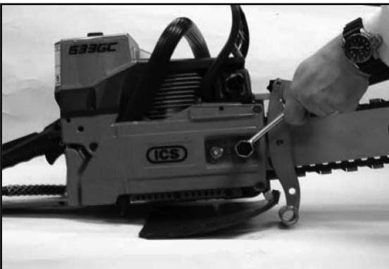
STEP 3 Tension bar and chain as described in the 633GC operators manual
