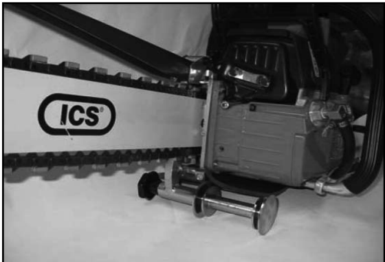
STEP 4 Insert axle into the mounting bracket as shown and firmly tighten knob
