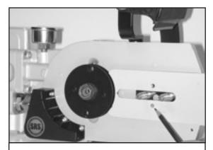
STEP 2 Place bar onto studs and chain adjustment pin.
