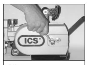
STEP 1 Loosen side cover nuts and remove side cover.
