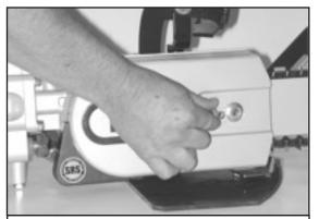
STEP 7 Install the side cover over the bar studs and install side cover nuts. Finger tighten only.
