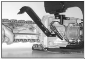
STEP 5 Make sure all of the drive links are inside the bar groove then pretension the chain.
