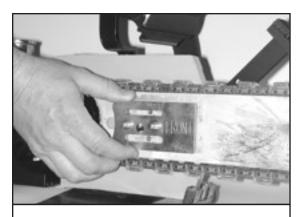
STEP 6 Install bar clamp plate over the bar studs.
