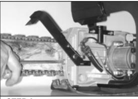
STEP 8 Tension the chain. The chain should be tight, but able to be pulled around the bar by hand (See Note 1).
