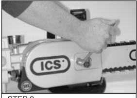
STEP 9 Lift up on the nose of hte bar and firmly tighten the side cover nuts (See note 2)
