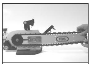
STEP 4 Mount the chain on the bar starting at the drive sprocket & continue over the bar nose.
