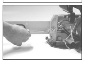
STEP 3 Turn chain-tensioning screw CCW until the bar comes into contact with the drive sprocket.
