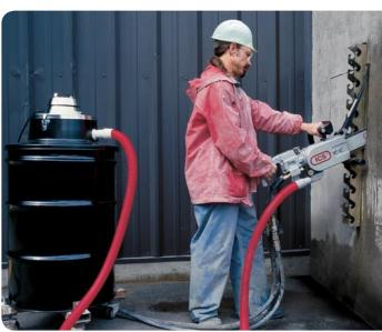
The TSS-55 Hi-Lift Performance Vacuum is designed to fit and seal on top of a standard 55 gallon drum without the use of any external fasteners or modifications.
