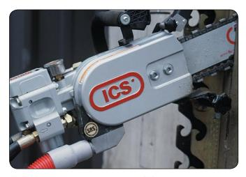
The TSS Vac-Attachment fits on to the 853 Pro saw to collect water and slurry while cutting.
