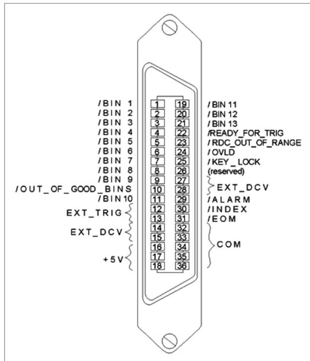
Figure 11. Pin assignment
