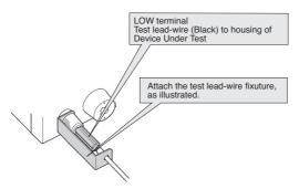
Fig.2-2 Connecting of test lead-wire on LOW side
