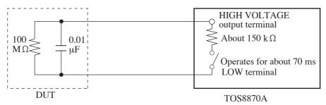
Fig.2-5 Example of discharge of equivalent circuit
