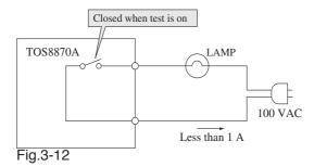
To obtain an "L" level digital signal with the contact signal.
