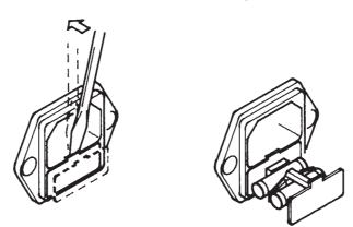
Figure 1-2 Removing the Fuse Holder
