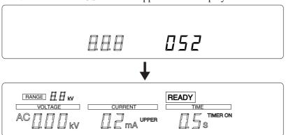
Within several tens seconds from the above, the initial test setup data will appear again.
