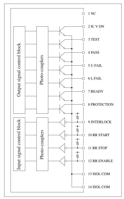
Figure 3-4 SIGNAL I/O Internal Configuration
