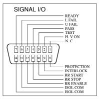
Figure 3-3 SIGNAL I/O Pin Configuration
