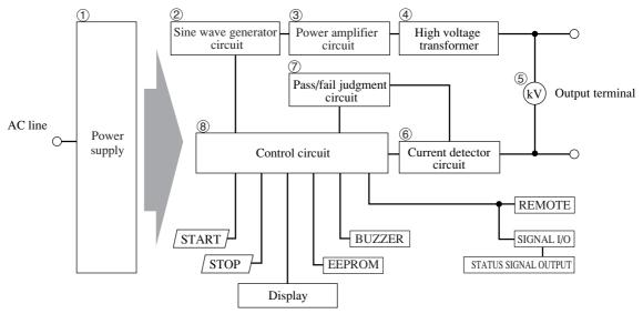
Figure 5-1 TOS5052 Block Diagram
