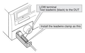
Figure 3-2 Connecting the low-voltage side test leadwire
