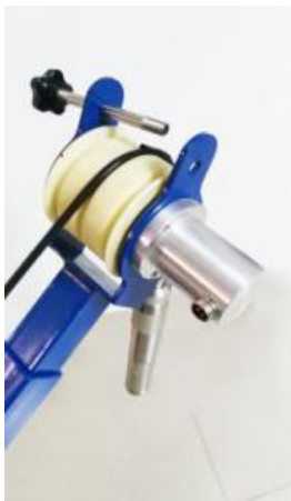
Loosen bolt and put into cable
