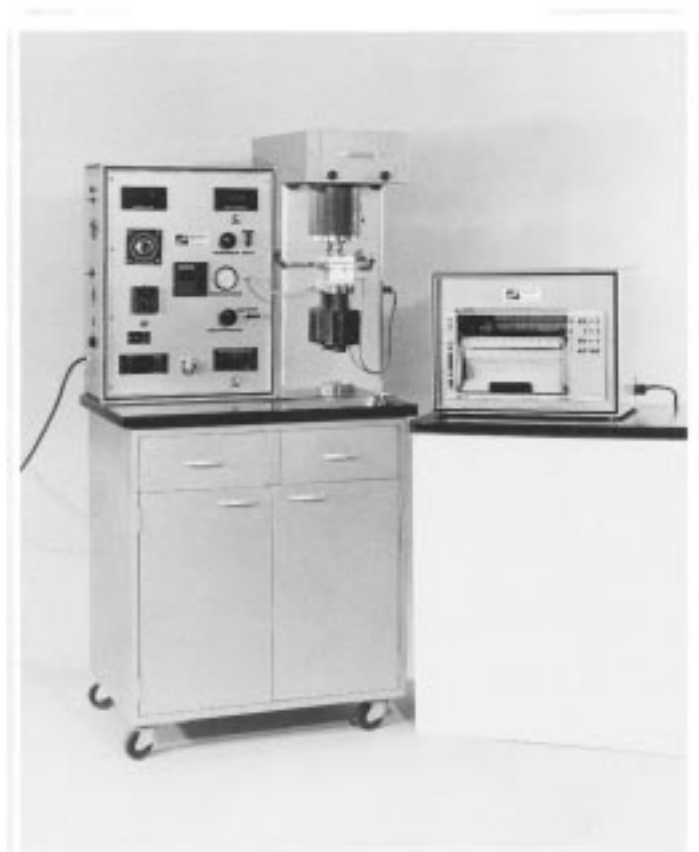
FIG. 3 Falex Variable-Speed Four-Ball Wear Test Machine
