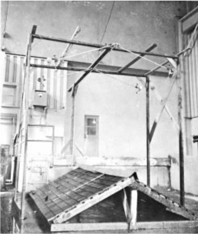
FIG. 1 Rain Test Apparatus Suitable for Method A
