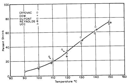
FIG. 5 Round Robin Data for Transverse-Direction Shrinkage of Biaxially-Oriented Polysulfone Sheeting
