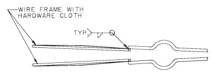
Note 1—Weld one wire frame to the inside of both arms of the tongs as shown. FIG. 2 Assembly of Specimen Holder
