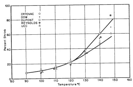
FIG. 4 Round-Robin Data for Machine-Direction Shrinkage of Biaxially-Oriented Polysulfone Sheeting
