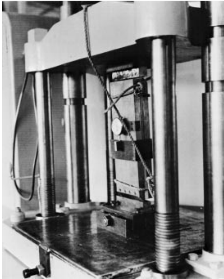
FIG. 3 Planar (Rolling) Shear Specimen Ready for Testing
