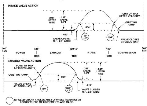
FIG. A4.1 Camshaft Timing Diagram
