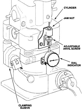
FIG. A4.3 Cylinder Height Dial Indicator
