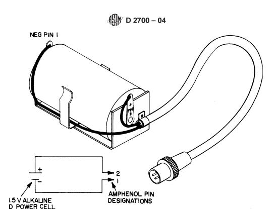
FIG. A3.2 Test Signal Source—Knockmeter Tracking Accuracy Check
