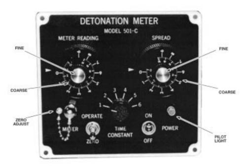
FIG. A4.7 Detonation Meter—Front Panel
