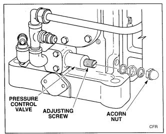
FIG. A4.8 Oil Pressure Control Valve Assembly
