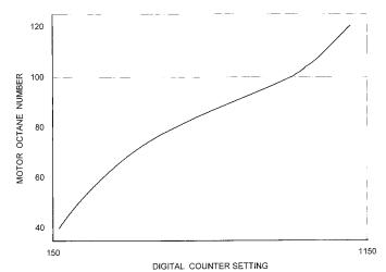
FIG. 3 Motor O.N. Versus Digital Counter Reading Characteristic
