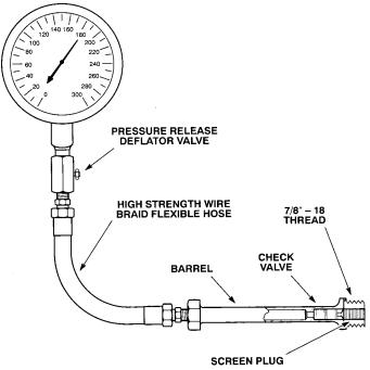
FIG. A4.4 Compression Pressure Gage Assembly
