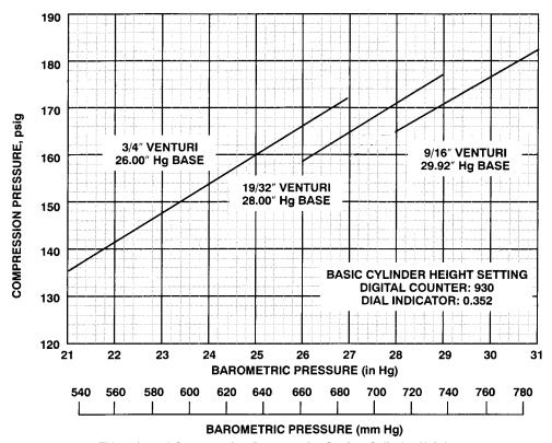
FIG. 2 Actual Compression Pressure for Setting Cylinder Height
