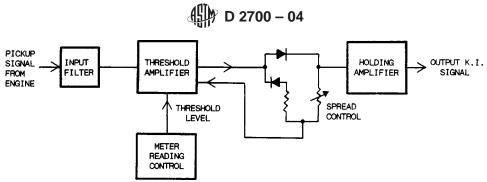
FIG. A4.5 Block Diagram of Knock Measurement System
