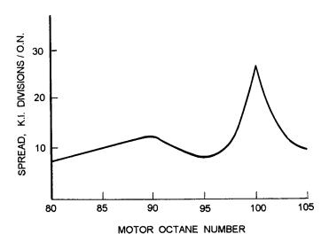
FIG. A4.6 Typical Detonation Meter Spread Characteristic
