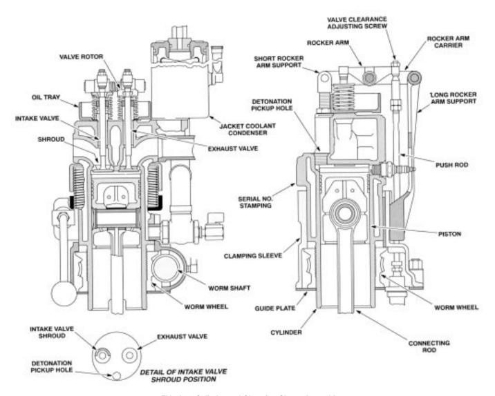
FIG. A2.2 Cylinder and Clamping Sleeve Assembly
