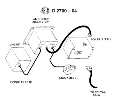
FIG. A3.1 Components of Knock Measurement Instrumentation
