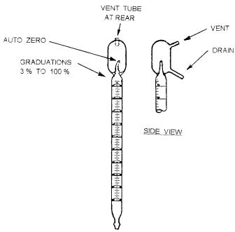
FIG. X1.1 Typical Reference Material Dispensing Apparatus-Single Buret Style
