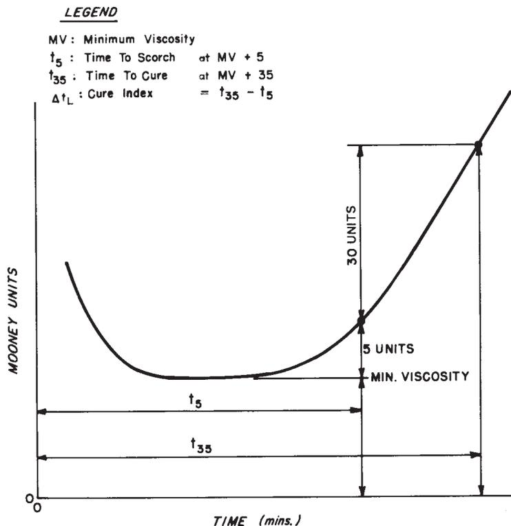
FIG. 4 Typical Prevulcanization Characteristics Curve Using Large Rotor
