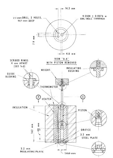
FIG. 1 General Arrangement of Extrusion Plastometer
