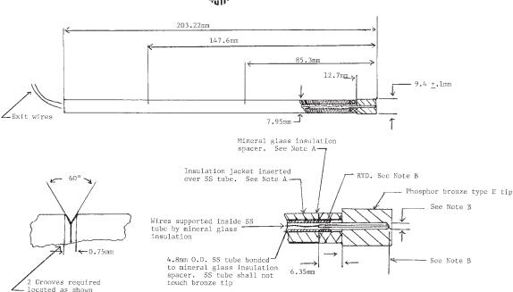
FIG. 3 Example of a Temperature Calibration Device
