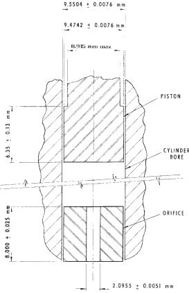
FIG. 2 Details of Extrusion Plastometer
