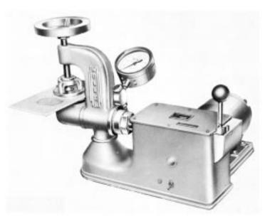
FIG. 1 Mullen Tester, Model A
