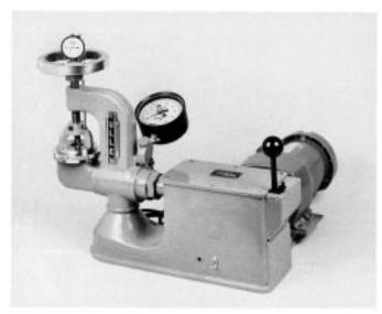
FIG. 2 Mullen Tester with Dial Gage
