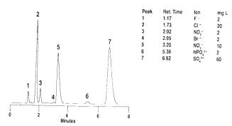
FIG. 1 Chromatogram Showing Separation Using the AS4A Column
