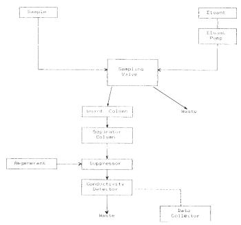
FIG. 2 Schematic of an Ion Chromatograph
