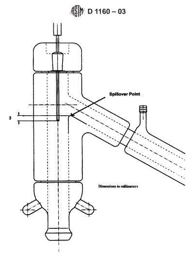
FIG. 8 Thermocouple Temperature Measuring Device
