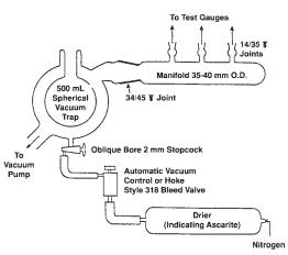
FIG. A3.1 Calibration of Vacuum Gages
