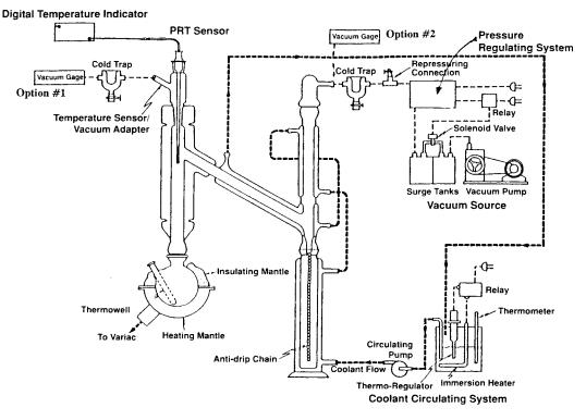
NOTE—A cold trap can be inserted before the pressure transducer in Option No. 2, if desired, or if the design of the transducer, such as a mercury McCleod gage, would require vapor protection.
