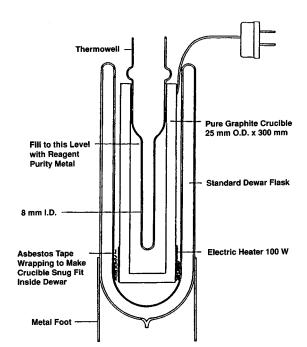
FIG. A1.1 Melting Point Bath for Temperature Standards
