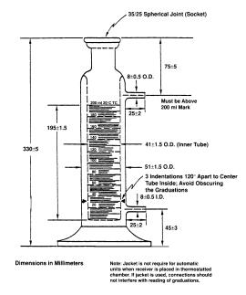
Note—Jacket is not required for automatic units when receiver is placed in thermostatted chamber. If jacket is used, connections should not interfere with reading of graduations.
