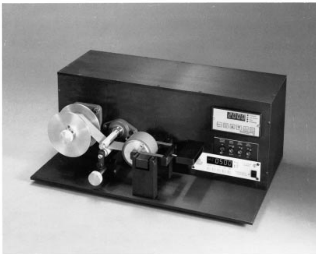
FIG. 3 Test Machine for Unwind Force Test (Method A)
