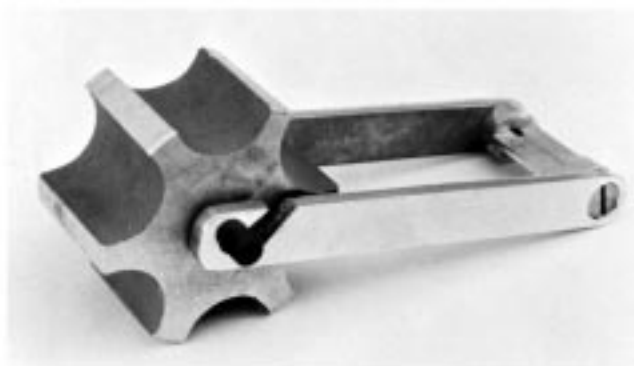
FIG. 4 Test Jig for Unwind Force Test
