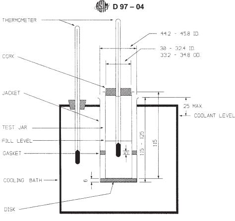
Note—Dimensions are in millimetres (not to scale). FIG. 1 Apparatus for Pour Point Test
