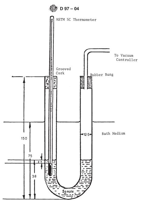
Note—All dimensions are in millimetres FIG. X1.1 Disposition of U-tube in Fluidity Temperature Test Bath
