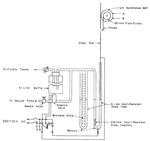
FIG. X1.4 Detail of Automatic Vacuum Controller
