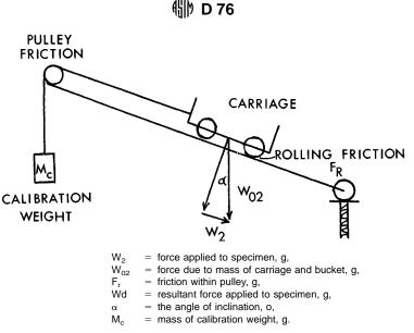
FIG. A1.1 Schematic of Applicable Forces
