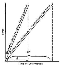
FIG. 1 Limitations on Response Speed of Recorder Pen
