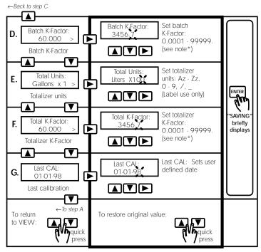
\*Note: Batch and totalizer K-Factor settings represent the number of pulses generated by the +GF+ SIGNET flow sensor for each engineering unit of fluid measured (published in the flow sensor manual).
