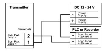
Example: Two transmitter connected to PLC/Recorder with separate power supply
