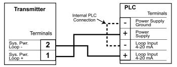
Connection to a PLC/Recorder, separate supply
