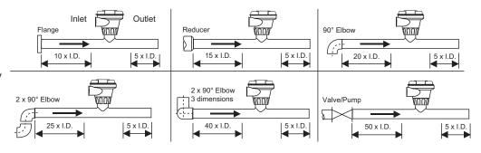
These configurations guarantee that the 2551 sensor will not be exposed to air bubbles when the system is in operation. These installations are recommended only if the system is designed to keep the 2551 sensor wet at all times.
