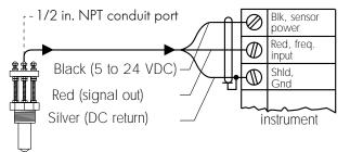
• Use 2-conductor shielded cable for cable extensions up to 300m (1000 ft.)
