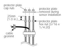
**F.** Thread protector plate hex nuts onto each of the three threaded rods. Adjust each hex nut to a height of approximately 25 mm (1 in.) from the top of each rod. Remove the black plastic cable grommet in top of sensor with a screwdriver. Slide the grommet up the cable away from sensor. (Fig. 12)
