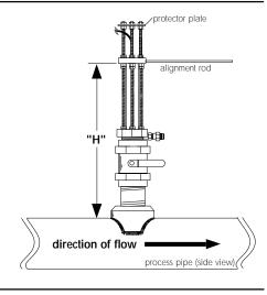
**D.** Place the alignment rod in the alignment hole on the sensor flange. Align the flange so rod is parallel to the process pipe. (Fig. 6)
