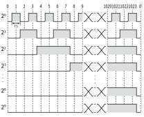
Parallel open collector output type multi-turn count (8192 revolution)
