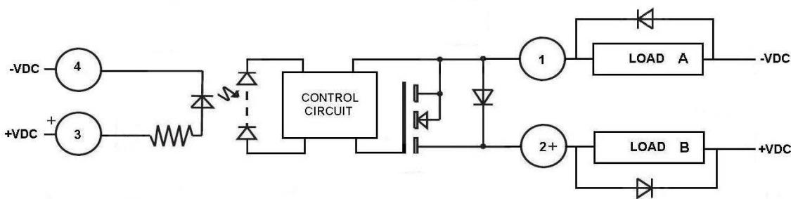
Load can be wired in position A or B
