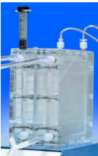
Two modules in parallel will concentrate 5 litres in under 75 minutes
