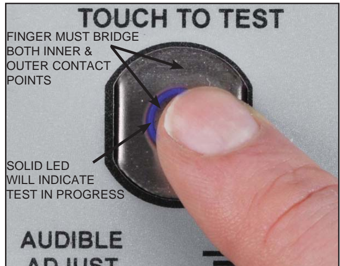
Figure 9. Bridge test contacts with finger
