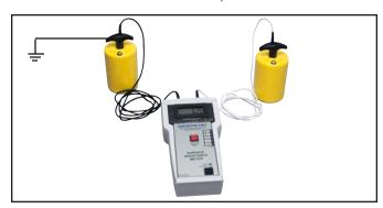
Figure 3. Setting up for RTG testing.
