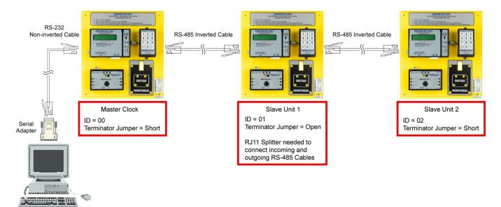
Figure 5. Connecting more than one SmartLog  $X^{3TM}$
