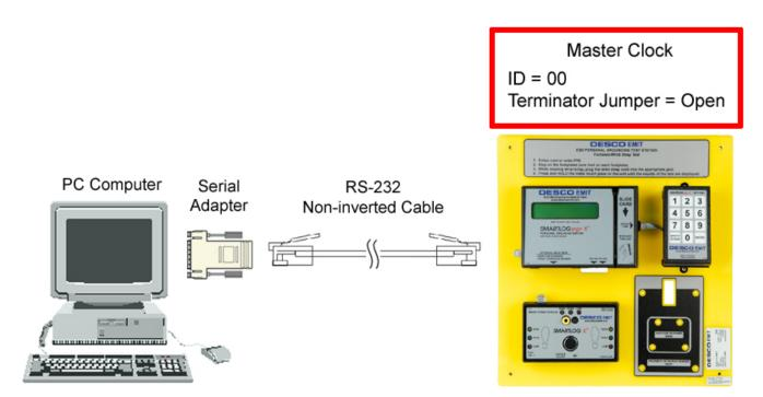
Figure 4. Connecting one SmartLog X<sup>3</sup>™
