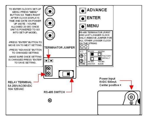
Figure 3. Back-side of SmartLog X<sup>3</sup>™ plate
