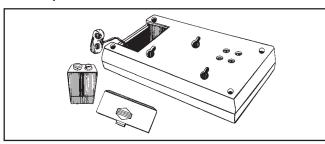
Figure 4. Replacing the battery
