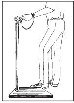
Figure 11. Testing of wrist strap grounding assemblies
