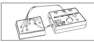
Figure 14. Calibration of the Combo Tester 750 Kilohm to 10 Megohm range with the model 07010
