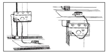
Figure 3. Stationary installation of the Combo Tester
