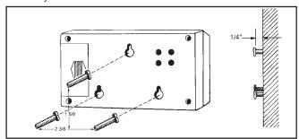
Figure 2. Mounting hole locations.
