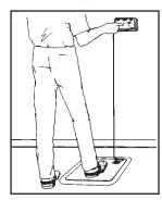
Figure 7. Testing foot grounding devices with 19253.
